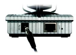
Figure 4-2: Connect the Power Adapter
